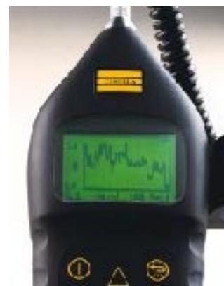
real time scrolling display of concentration levels with user selectable time bases and auto ranging y-axis scale
